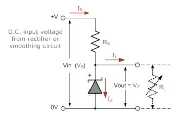
A 20.0V stabilized power supply is required to be produced from a 24V DC power supply input source. The maximum power rating  $P_Z$  of the zener diode is 4kW. Using the zener regulator circuit above calculate.
