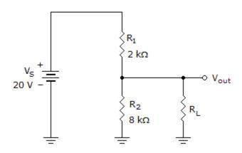
If the load ( $R_L$ ) in the given circuit is 120 k $\Omega$ , calculate the loaded output voltage?
