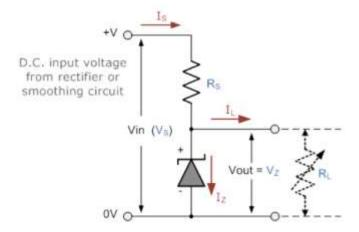
A 5.0V stabilized power supply is required to be produced from a 12V DC power supply input source. The maximum power rating Pz of the zener diode is 2W. Using the zener regulator circuit above calculate.
